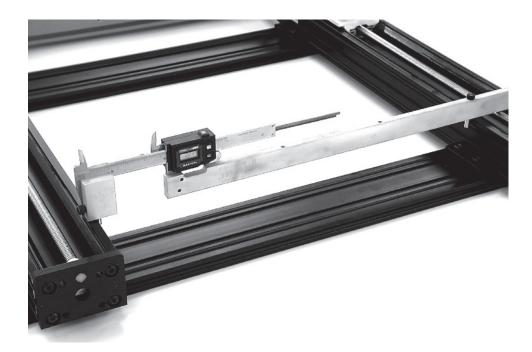
Loosen the mounting cleats on the driven slide nearest to the pulley end. Place the belt tensioning rod between the motor mounting plates of both slides and tighten until the rod will support it's own weight.
