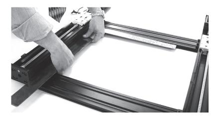
$\overline{7}$  Tighten the mounting cleats on the drive (motor) side.
