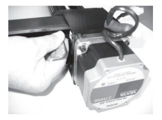
**CAUTION** Never remove Motor or Idler cover plate when belt is in tension, Severe damage to Pulley Shaft and Leadscrew will occur!
