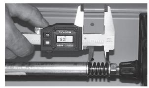
Check for parallel between the two slides and adjust the driven slide as necessary. Recheck the change in spring length. Periodically rotate the belt to ensure correct belt seating. **NOTE**: The slides should be parallel within 0.002" for proper slide operation. Use a cross pattern tightening sequence on the mounting cleats after final check.
